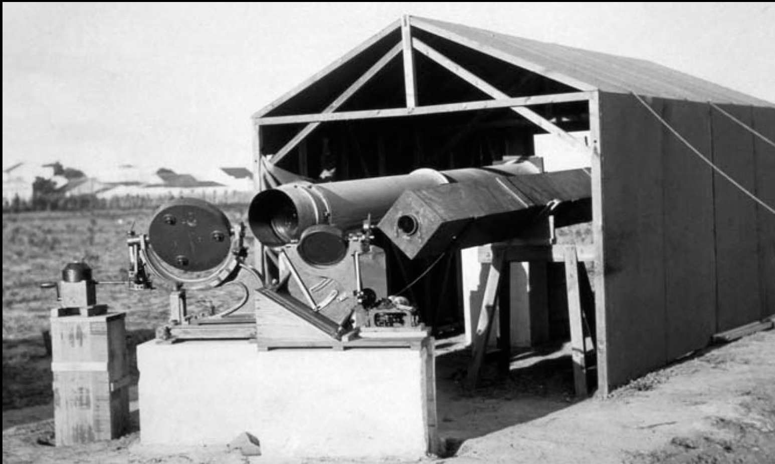
Instruments at Sobral, Brazil. The 4-inch lens is in the square tube on the right, and the astrographic lens, chosen for its wide field of view, is in the circular tube on the left. In front of the tubes are mirrors that are driven by a mechanism that keeps the stellar images at the same position on the plates during an exposure. The mirror on the left was the chief suspect in the poor-quality astrographic-lens images produced during the 1919 eclipse.
